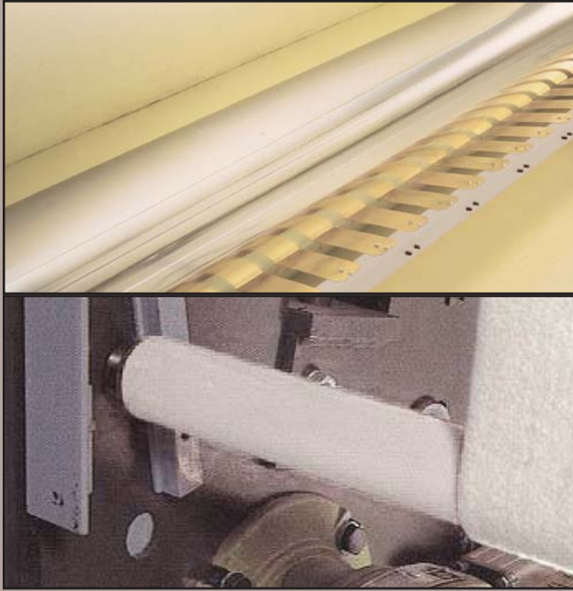
Top photo: The cylinder is made in machined steel, mirror polished and finished in chrome. Bottom photo: Kinematic strap tensing system ensures optimum ironing quality.
